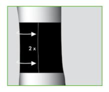
Wrap the ArboTape wound sealer around the tree (1-2 times). The wound surface must be sealed to prevent dehydration.
