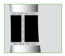
4 Fix the ArboTape by using the Bio-Tape organic fixing tape.
