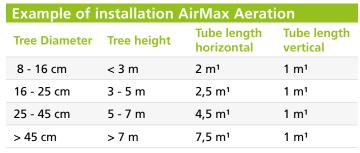
Ø Tube horizontal: 80 mm Ø Tube vertical: 80 mm
